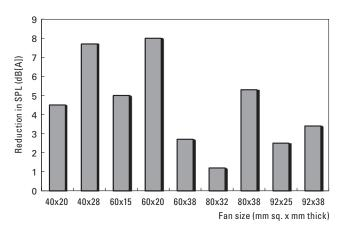
Fig. 4: Reduction in SPL from conventional models
