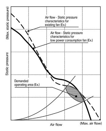
Fig. 1: Comparison of characteristics for existing and low power consumption fans
