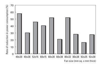
Fig. 3: Rate of reduction in power consumption from conventional models
